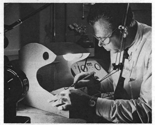
POST-MORTEM INSPECTIONS of defective components are part of the job performed by Quality Engineering Department 2120. Such investigations demand care and skill, as well as frequent use of unusual equipment. W. D. Harwood of Component Evaluation Section B, 2123-2, uses dental drill to search for reasons of defect found in component under test.
